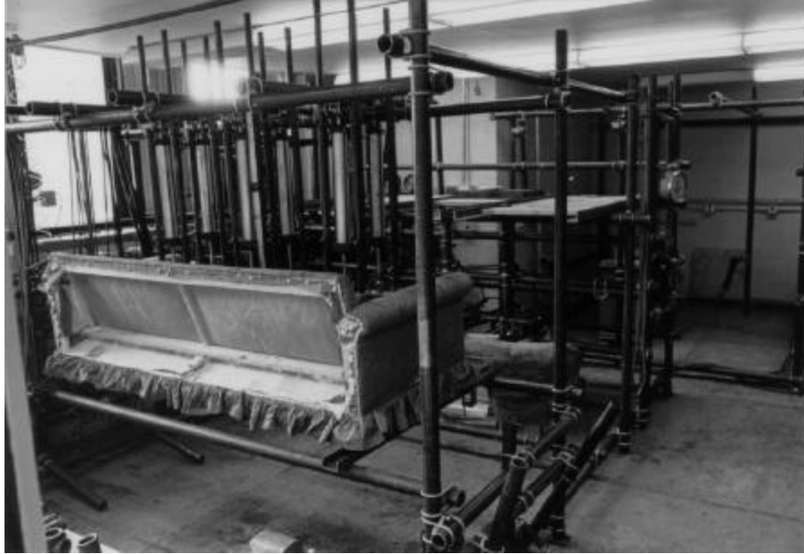
Figure 1. Typical main testing machine framework in which the specimens are placed for testing.
