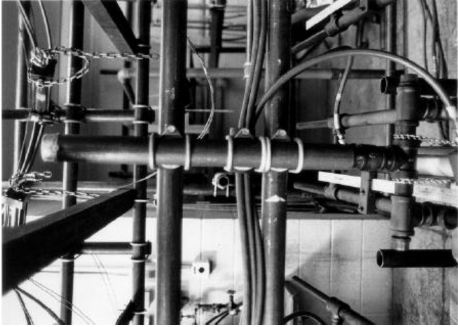
Figure 12. The vertical external 2 inch diameter swivel sleeve bearing provides a means of attaching the backrest load frame to the main testing machine frame. The inner 1-1/2 inch diameter swivel column is free to rotate within the external sleeve bearing. This allows the backrest load frame to swivel from side to side as well as pivot up and down. As a result, the load frame is able to follow complex movements of the backrest as it deflects under load.
