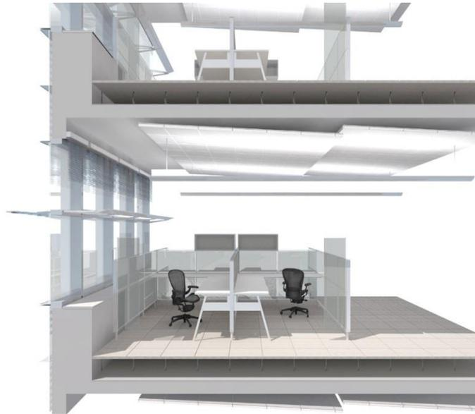
Floors 1–3 use a traditional overhead-delivery HVAC system. Floors 4–9 (office spaces) are conditioned through a UFAD system (Figure 4-5). Under-floor systems offer several advantages:
