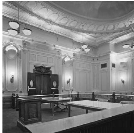
FIGURES 5-6 GSA Building Preservation Plans identify spaces of architectural importance and character-defining features to be preserved and restored, such as this hidden ornamental ceiling restored as part of the building systems upgrade.
