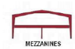
RIGID FRAME Low Profile with by-pass girts
