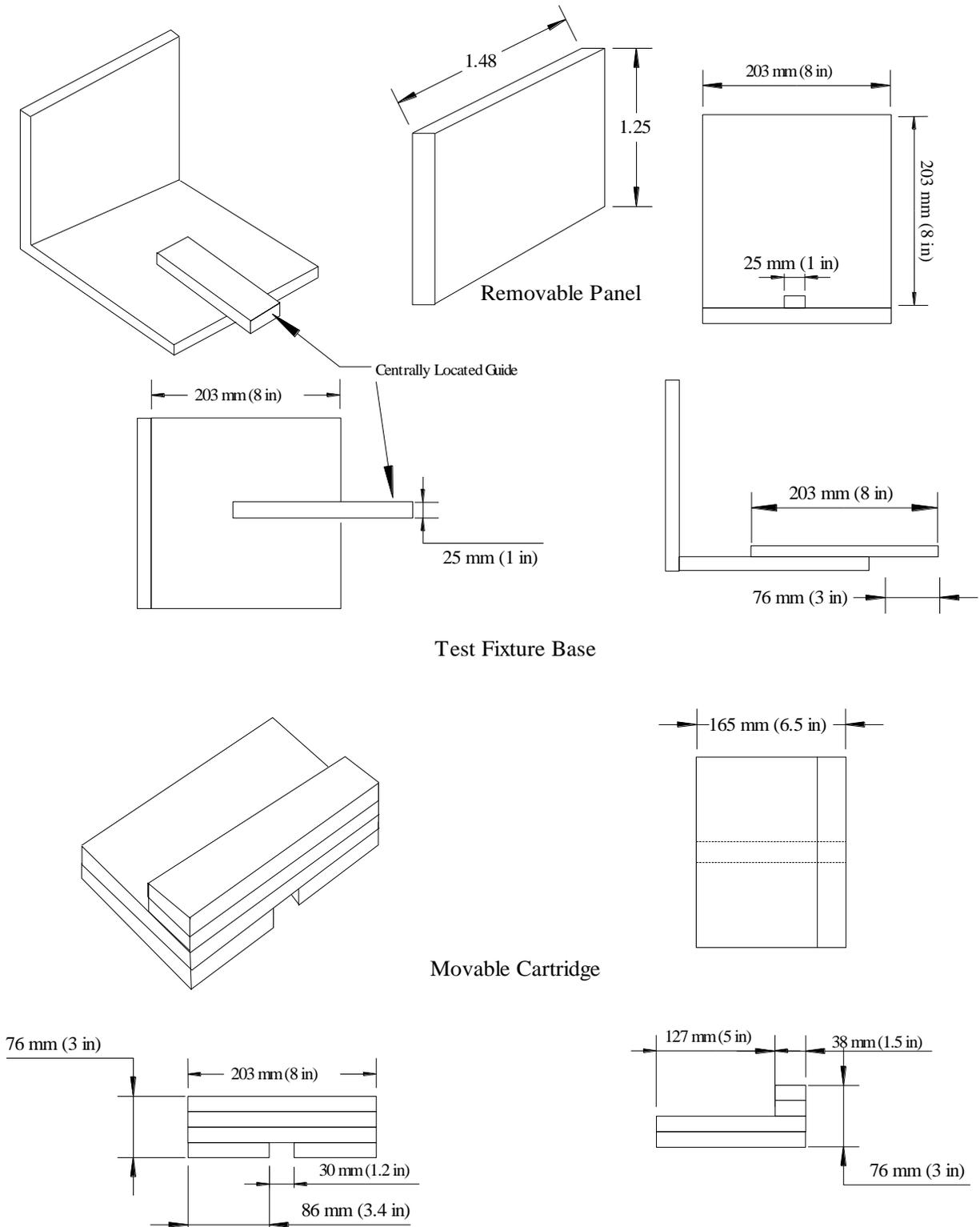
Figure C-2. Mock-up Assembly for Smoldering Ignition Resistance Test of Upholstery Cover Fabrics
