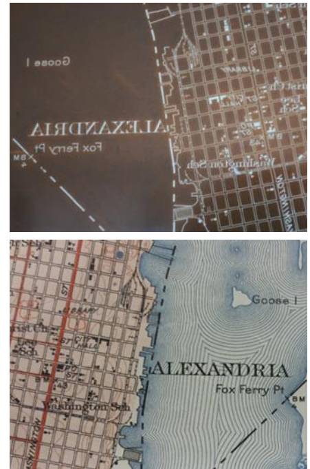
Figure 1. A portion of an engraving (top) used to print the black ink for a USGS topographic map (bottom). (Photo courtesy of Bruce Geyman, USGS.)
