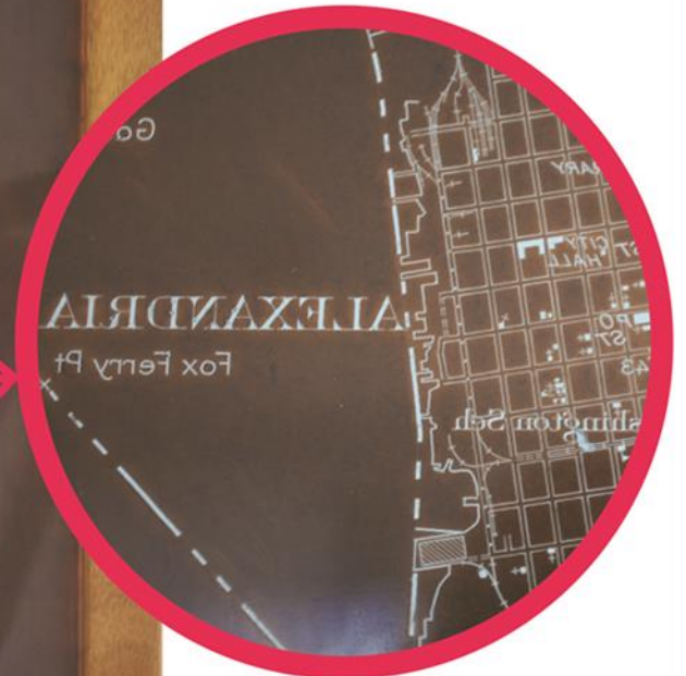
Figure 3. (Left and above) Close up of the engraving used to print cultural, transportation, and boundary features and text with black ink. The inset shows the mirror-image reversal of the point and line symbols and text. The engraved symbols and text have been enhanced by coloring them white to improve their visibility for display. (Image courtesy of Bruce Geyman.)
