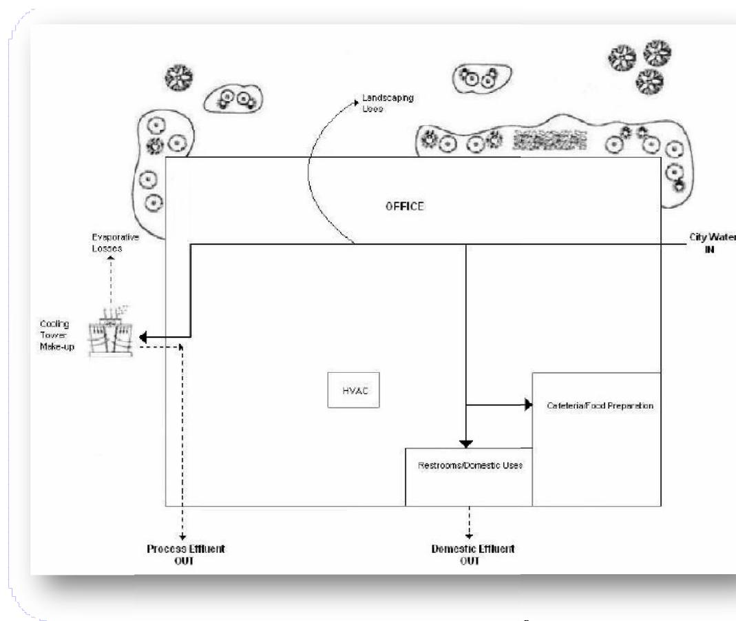
Figure 3: Sample Water Balance Diagram<sup>6</sup>
