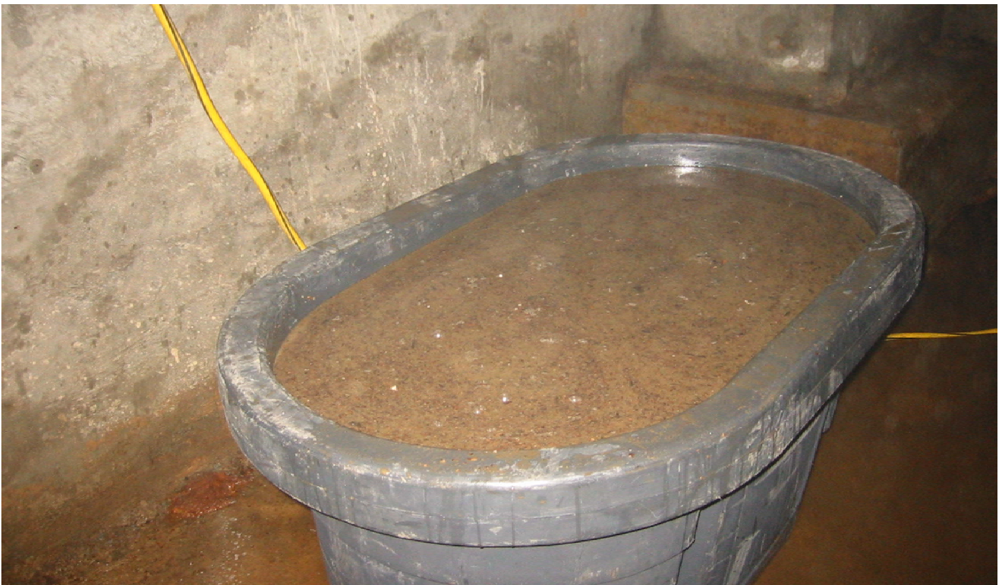
Photograph 34. Building 105 SAFR. Rinsate after 50 micron filtration and before 0.5 micron filtration, September 2002.
