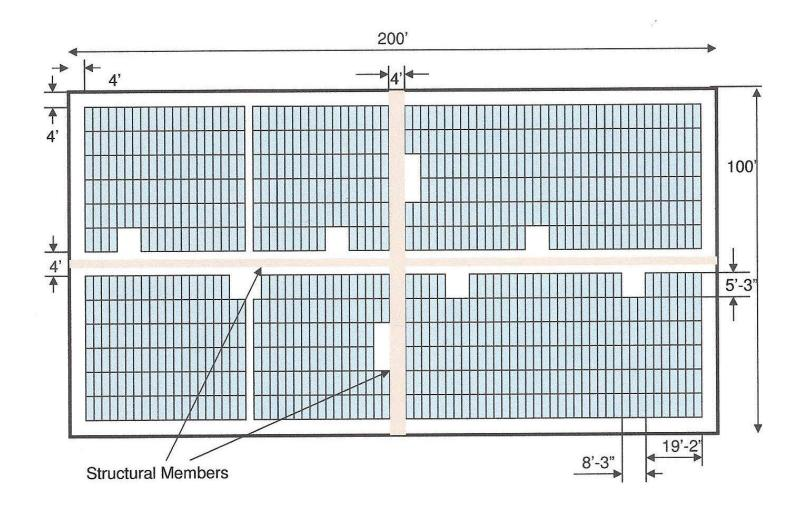
Figure 2. PV Array Example: Small Commercial Building (Axis > 250 ft.). 4 ft. walkways
