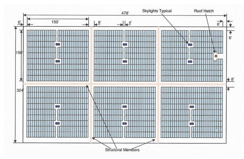
Figure 1. PV Array Example: Large Commercial Building (Axis > 250 ft.). 8 ft. walkways
