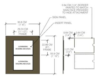
Figure 6.27 Temporary message sign panel detail.
