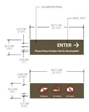
Figure 6.25 Security equipment signs detail.
