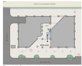
Figure 7.20 Plan of the existing building showing the hourglass shape of the lobby and the setback from the sidewalk. The setback of the entrance from the street compresses the security station into the middle of the lobby, creating a situation where people in the midst of the security process occupy the same space as people using the elevators.
