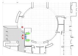
Figure 7.39 The design creates layered spaces for queuing and screening. A smaller free zone results in a more generous lobby.
