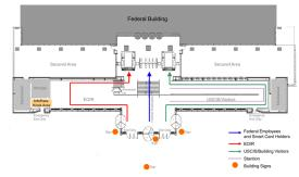
Figure 7.01 The security design creates three separate paths of circulation for Federal employees, EOIR, and visitors, and places the free zone entirely outside the perimeter of the original building.
