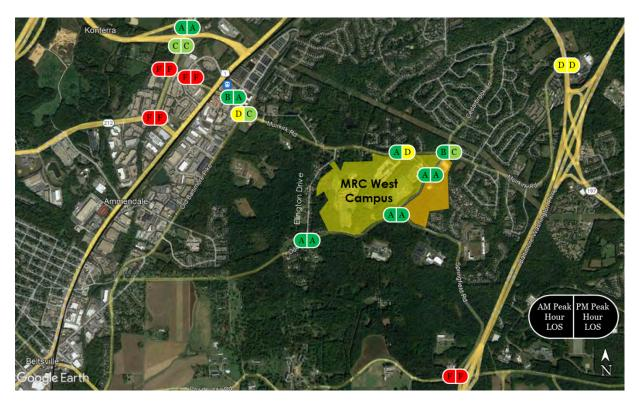
Figure 14: Phase 2 Action Condition (Alternatives A & C) Overall Intersection LOS
