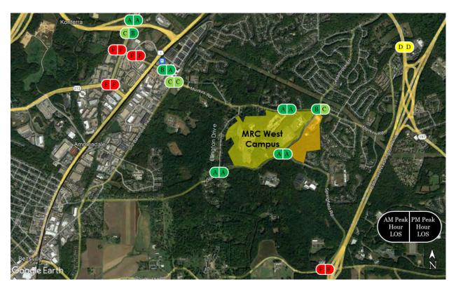
Figure 11: Phase 2 No Action Condition Overall Intersection LOS
