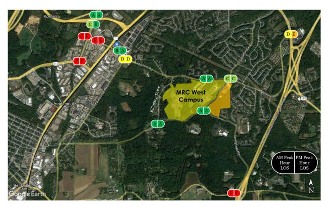
Figure 12: Phase 3 No Action Condition Overall Intersection LOS
