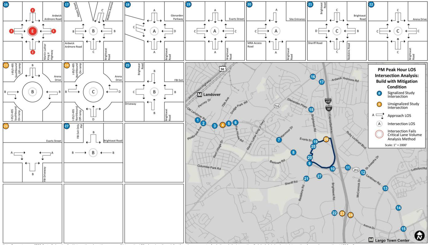
Note: One- or two-way STOP-Controlled unsignalized intersections do not have an overall intersection LOS value, since the mainline through move operates freely through the intersection. Red shaded circles denote intersections/approaches operating at LOS E or F.
