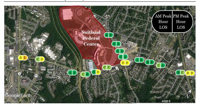
Figure 7: 2022 Build Condition Overall Intersection LOS
