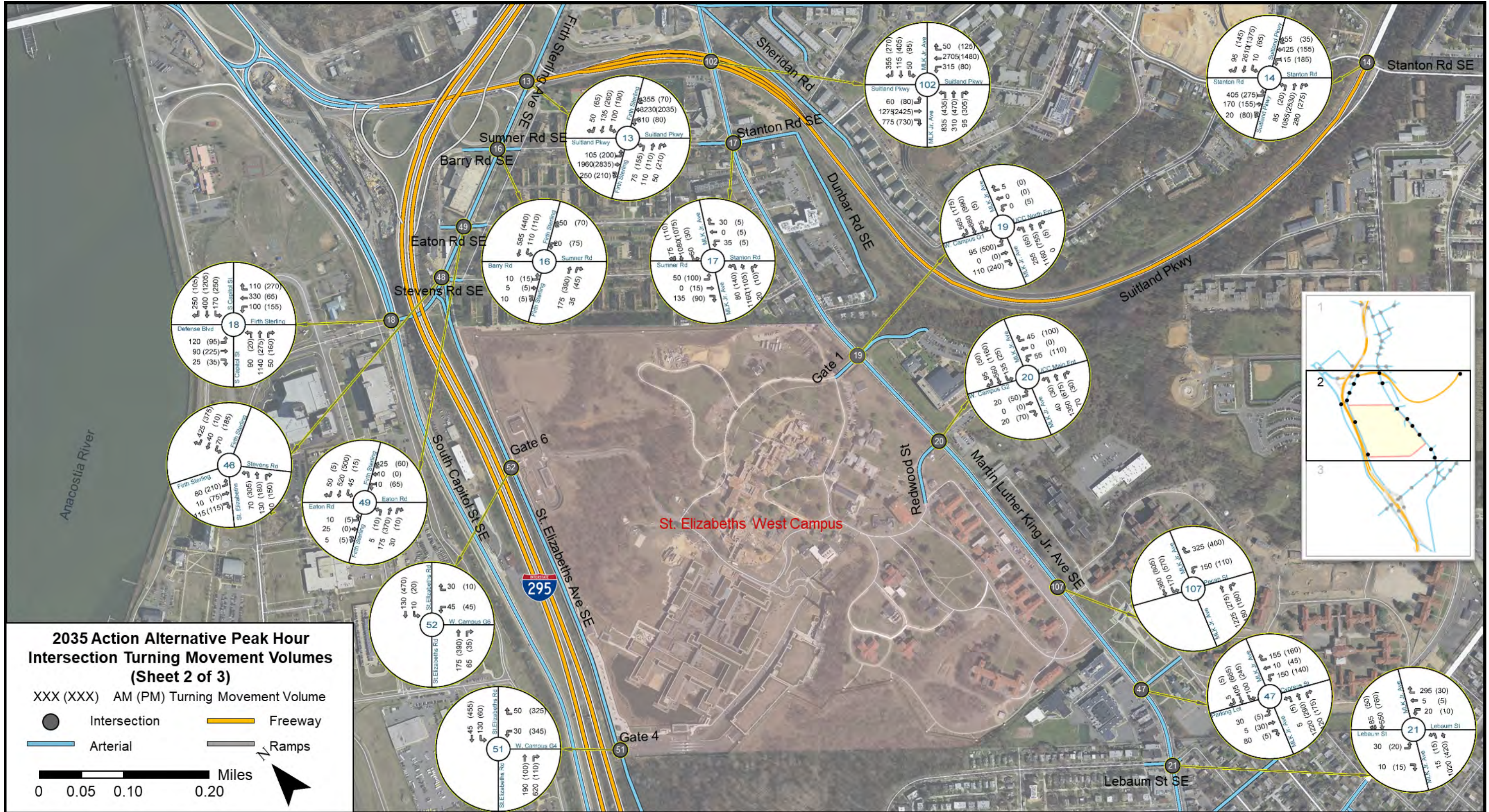
Figure 6-10: 2035 Action Alternative Intersection Turning Movement Volumes during AM and PM Peak Hours (sheet 2 of 3)
