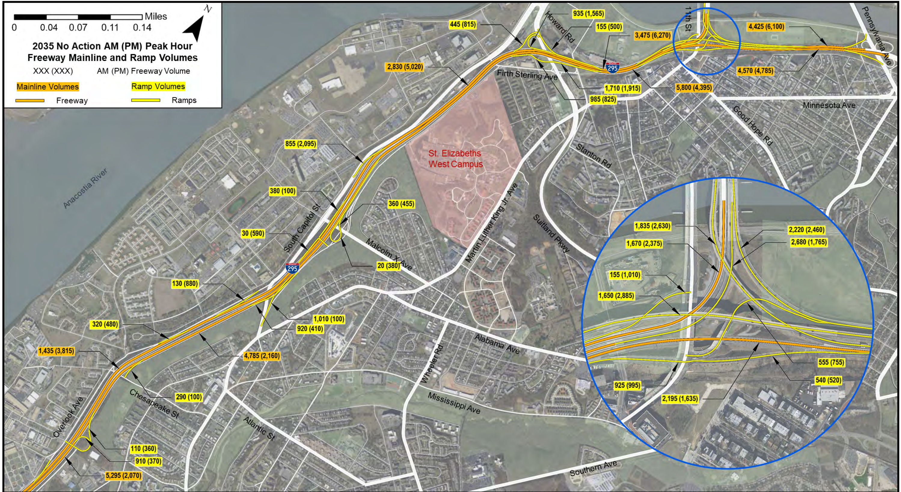
Figure 6-4: 2035 No Action Alternative Freeway Mainline and Ramp Volumes during AM and PM Peak Hours
