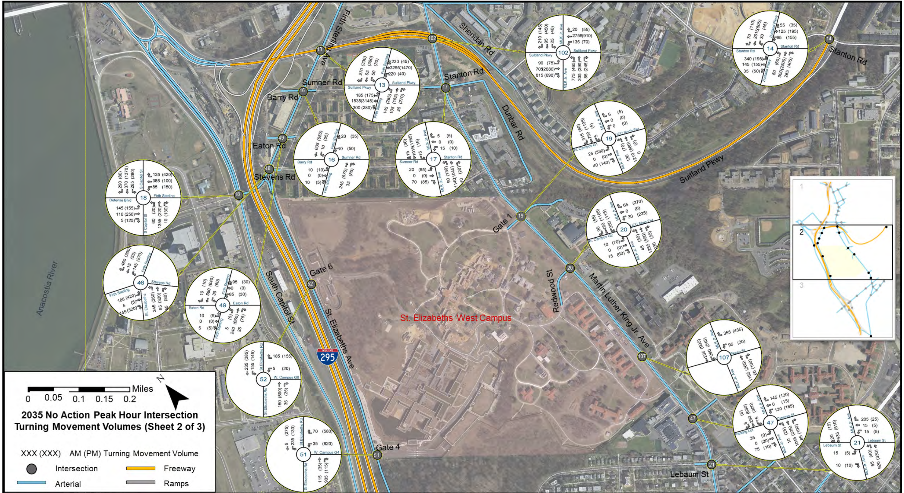
Figure 6-6: 2035 No Action Alternative Intersection Turning Movement Volumes during AM and PM Peak Hours (sheet 2 of 3)
