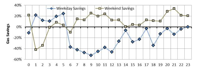
Overall, there was an average 4.8% decrease in natural gas consumption during all unoccupied when hours weathercomparing the corrected natural gas use in the baseline period to actual natural gas use during the study period. However, this was more than offset by an average 35.6% increase in consumption during
