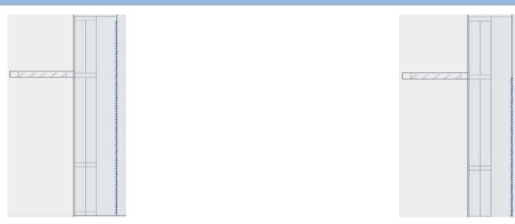
Figure 40 Building 9420 open office section (left) with the blind head height at the top of the vision glazing (right)
