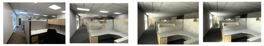
Figure 41 Open Office Image (top left) and Radiance Renderings of base case blinds closed (top right), full blinds partially open (bottom left), and vision glazing blinds only (bottom right)
