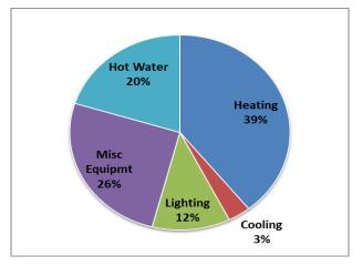
Figure 9 Barracks energy end-use breakdown
