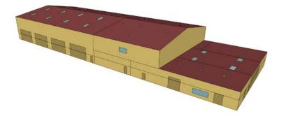
Figure 8 Tactical Equipment Maintenance Facility (TEMF) model (WWR=1%, SRR=3%)
