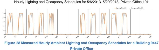
Hourly lighting and occupancy profiles for the monitoring period, shown in Figure 29 are meant to convey the highlevel trend that ambient electric lighting is used when the spaces are occupied. Offices 101 and 106 are interior offices and office 119 is a perimeter office. Each office type has daylighting features yet the natural resource is not resulting in
