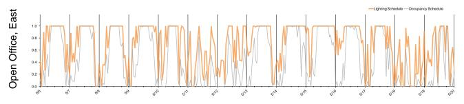
Figure 35 Measured Hourly Ambient Lighting and Occupancy Schedules for a Building 9447 High-Bay Module
