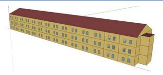
Figure 4 Barracks model (WWR=9%, SRR=0%)
