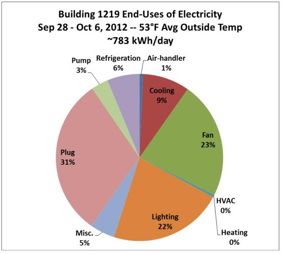
Figure 77 End-use energy consumption for Building 1219
