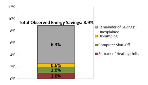
Figure 70 Total Observed Energy Savings in Building 1118 between Baseline and Intervention Period
