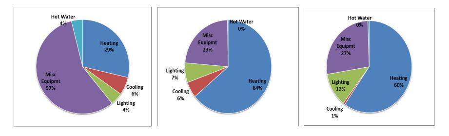
Figure 11 DFAC energy end-use breakdown
