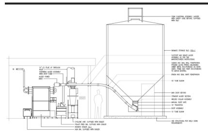
**Biomass Boiler and Fuel Bin** Wood pellets are stored in a silo outside of the building and are augured into the building on demand.<sup>2</sup>
