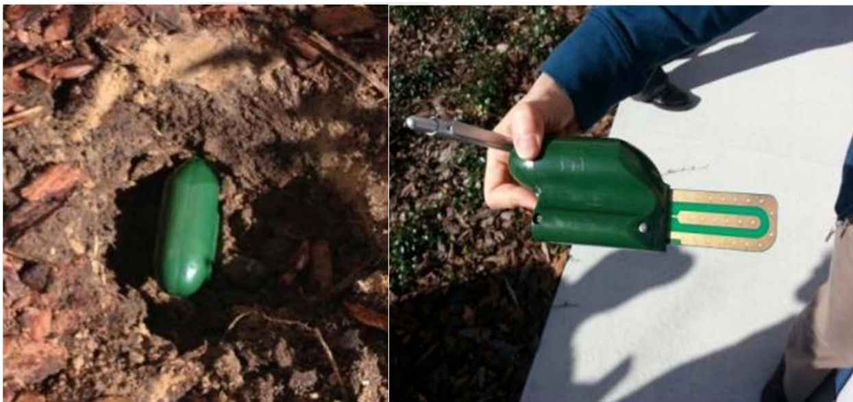
Figure 7. Photos of Soil Moisture Sensors
