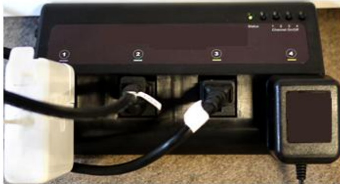
Figure IV-2: Image of a deployed APS in a GSA Office. Four devices are plugged in to the APS. The power strip is mounted on the desktop for easy user access. Credit: Enmetric Systems Incorporated
