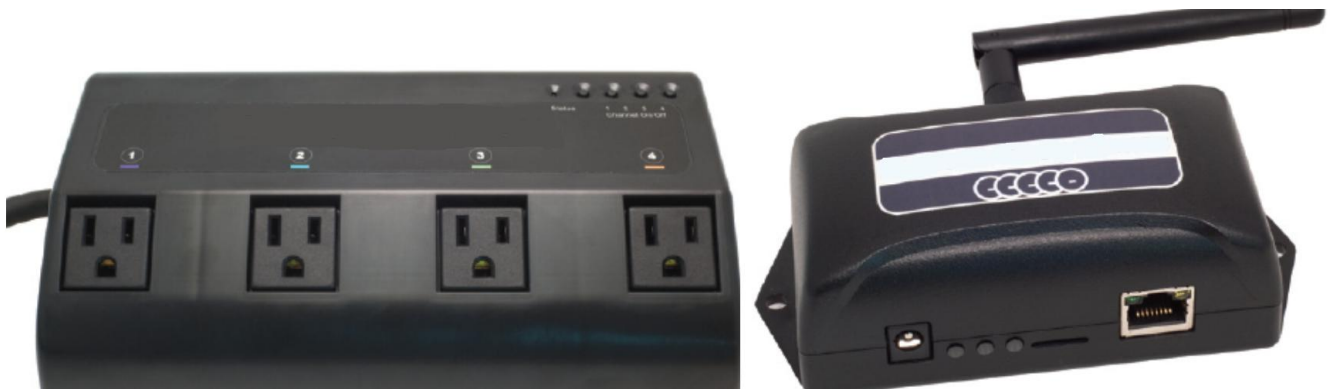
Figure IV-1: APS (left) and communications bridge (right). Credit: Enmetric Systems Incorporated
