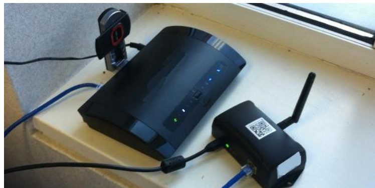
Figure IV-3: Image of wireless communication system. A wireless bridge and the cellular modem are shown here next to a window for optimum cellular reception. Credit: Ian Metzger, NREL
