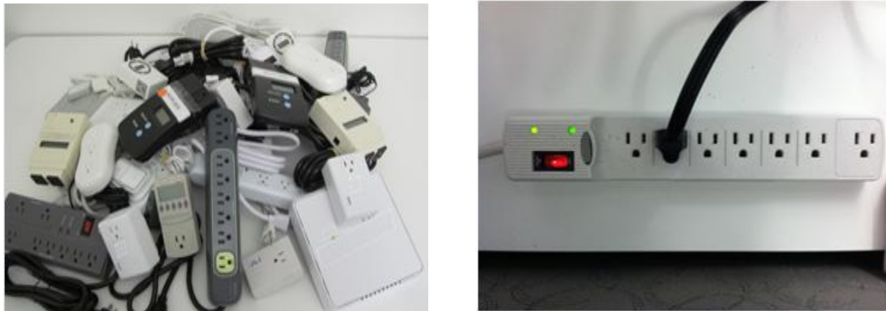
Figure VI-1: An example set of advanced plug strips that is currently on the market (left) and incumbent technology: standard no-control plug strip (right). Credit: Chad Lobato and Ian Metzger, NREL
