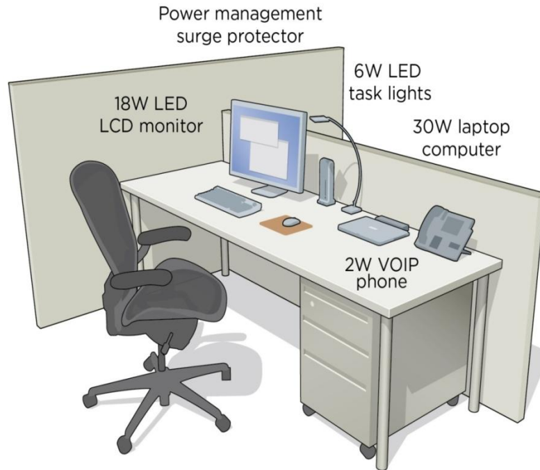
Figure VI-2: Example of low-energy workstation recommended as best practice. Credit: Mathew Luckwitz, NREL
