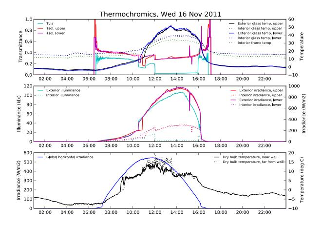
Figure 8: Thermochromic window switching pattern on a cold, sunny day (November 16, 2011). Thermochromic in this case switches to tinted from noon until 16:00 ST as indicated by the light blue line (Tvis') in the top graph.
