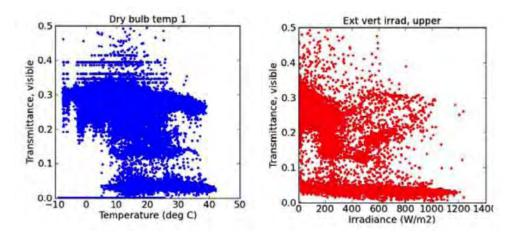
Figure 10: Nominal visible transmittance (Tvis') of the thermochromic window as a function of outdoor dry bulb temperature (left) and incident vertical irradiance (right).
