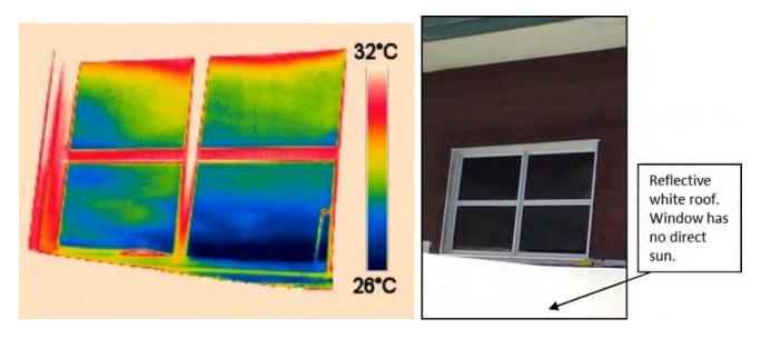
Figure 19: Infrared image (left) and photographic image (right) showing the thermal surface temperature patterns matching the switching pattern of thermochromic glazing when direct sun has not yet covered the upper panes. Images given for September 23, 2011, 11:03 AM ST.
