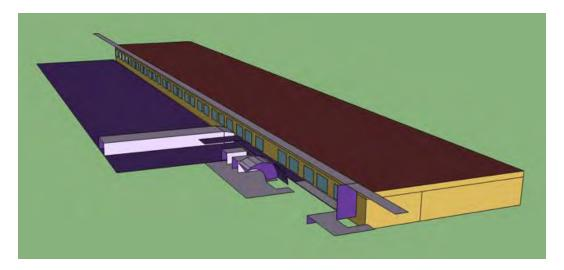
Figure 5: Schematic view of the modeled zone that was used as input to the EnergyPlus simulations. (The colors are not an indication of the actual color of the surfaces – they simply depict the different planes of the surfaces.)
