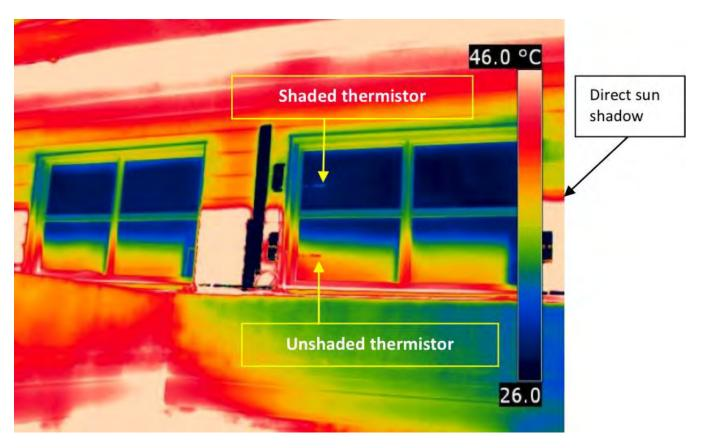
Figure 12: An infrared image of the dark tinted regions in the lower panes as the thermochromic transitions from clear to tinted with direct sun patches on the window. Image taken September 22, 2011, 11:57 AM ST.
