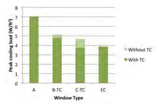
Figure 21: Peak cooling electricity use for single-pane clear (A), window with and without TC film (B-TC), low-e with and without TC film (C-TC), and electrochromic window. Results given for the 48-ft deep west-facing perimeter zone in the Denver Federal Center, Denver, CO.
