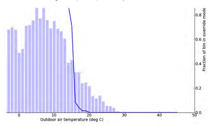
Figure 29: The amount of time that the outdoor air temperature was within a specific temperature range (bars shown in 1°C increments, left y-axis) and the percentage of that time that the Phase I control system was in the HVAC mode (line on the graph, right y-axis).
