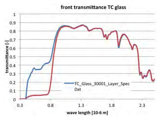
Figure 6: Solar transmittance for the thermochromic film on 6 mm clear glass. Solar transmission is shown with the dark blue line in the clear state (top) and the red line in the tinted state (bottom).
