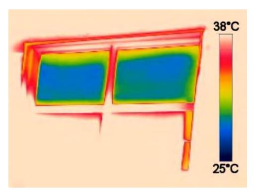
Figure 16: Infrared surface temperatures, no direct sun on the upper panes. Image taken September 22, 2011, 12:20 PM ST when the outdoor air temperature was 26°C.
