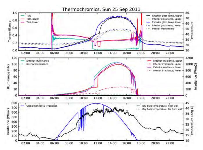
Figure 7: Thermochromic window switching pattern on a warm, sunny day around the autumnal equinox (September 25, 2011). Notice how in the upper graph (light blue line), the visible transmittance (Tvis) drops abruptly from a value of about 0.30 to 0.03 after around 11:00 in the morning. Time of day is shown on the x-axis (Mountain Standard Time). Nominal visible and solar transmittance data (Tvis', Tsol') are given on the
