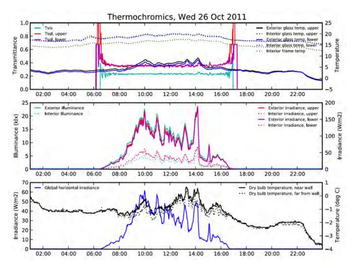
Figure 9: Thermochromic window switching pattern on a cold overcast day (October 26, 2011). In this case, the thermochromic window stays unswitched throughout the day as indicated by the light blue line (Tvis') in the top graph.
