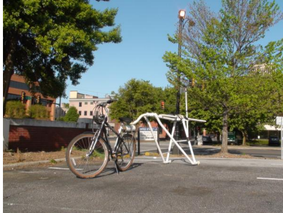
GEM-2 EM unit rigged for use with bicycle
