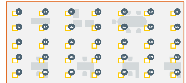
Figure 16 LLLC Systems Embed Sensors in Individual Fixtures
