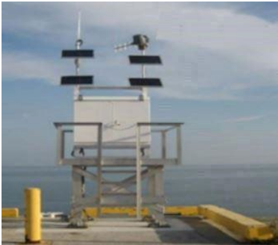
Photograph STR-1: This photograph is an example of tide monitoring station.
