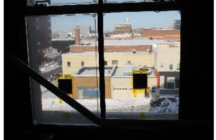
Window with heat flux sensors installed.
